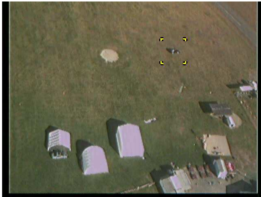
Figure 2. An example frame from the execution of our visual tracking algorithm run on a live UAV video stream, in this case tracking a car near a road. The centroid of the yellow corners is the current location of the object of interest.
