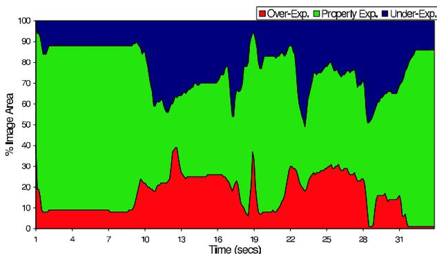
Fig. 5. Graph showing the limitations of a single exposure with a generic exposure control algorithm. At times there is only 20% correctly exposed area in the image. Graph of: over, under and properly exposed areas of our *regular* exposure.
