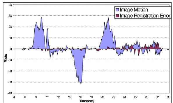
Fig. 7. Horizontal image motion of neighbouring exposure sequences. The motion is calculated by manually aligning the images. Also shown is the corresponding error of the automatic registration process.
