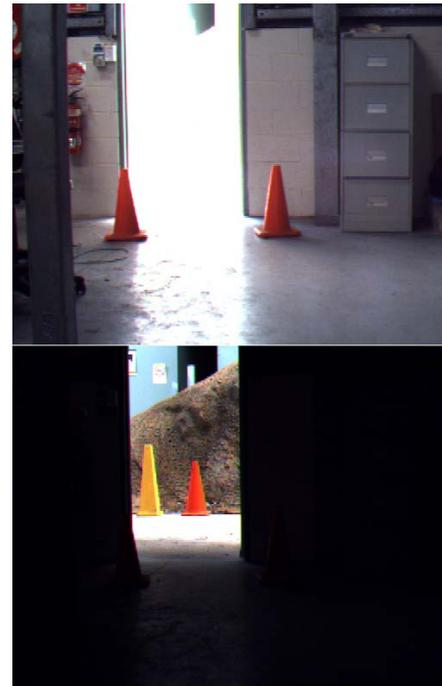
Fig. 1. Example showing the limitations of conventional LDR cameras. Top: Image taken with a regular exposure, areas outside are completely overexposed. Bottom: Image of the same scene taken with a short exposure, areas inside are completely underexposed.
