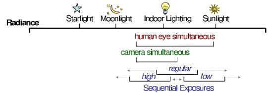
Fig. 2. Example illustrating natural radiance levels compared with the simultaneous radiance range of the human eye and that of a camera. Also shows the extended range of the sequential exposure technique. Rough estimates of range taken from [10], [1]
