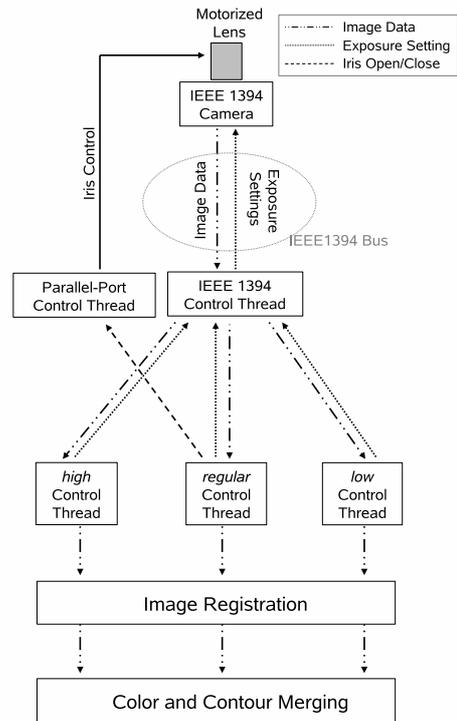
Fig. 3. Diagram of the overall system. Showing automatic control of the three sequential exposures and the lens aperture followed by image registration and merging.
