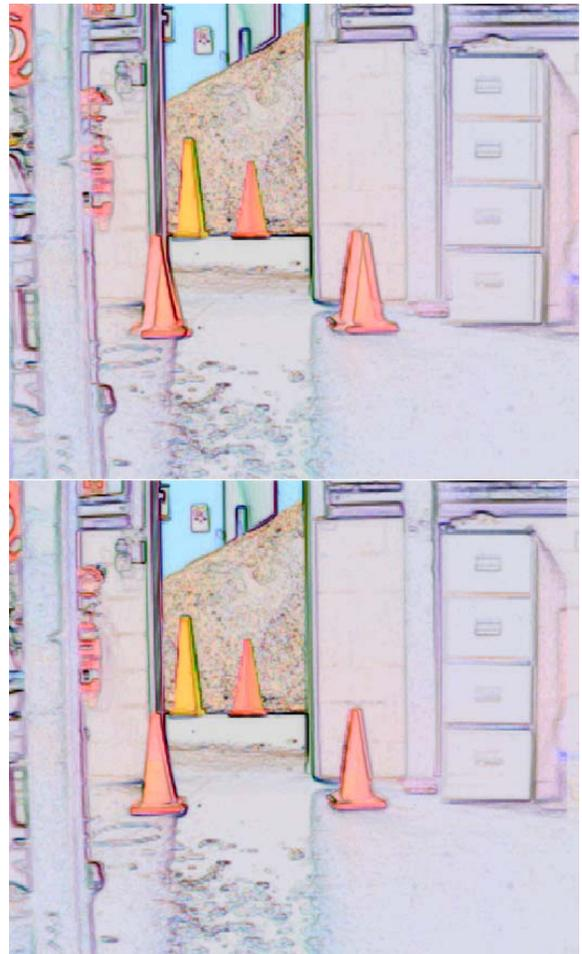
Fig. 8. Top: Merged sequence of exposures without registration. Notice the artifacts at the fire hose (top-left), traffic cones (centre) and drawers (right). Bottom: Merged sequence of exposures with automatic real-time registration and interpolation.
