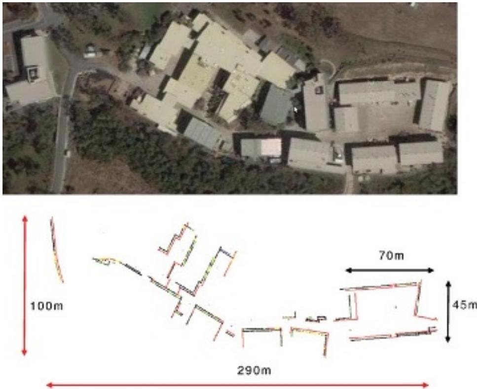
**Figure 2.** Top: Aerial image of the site. Bottom: Overhead view of the survey of the buildings.
