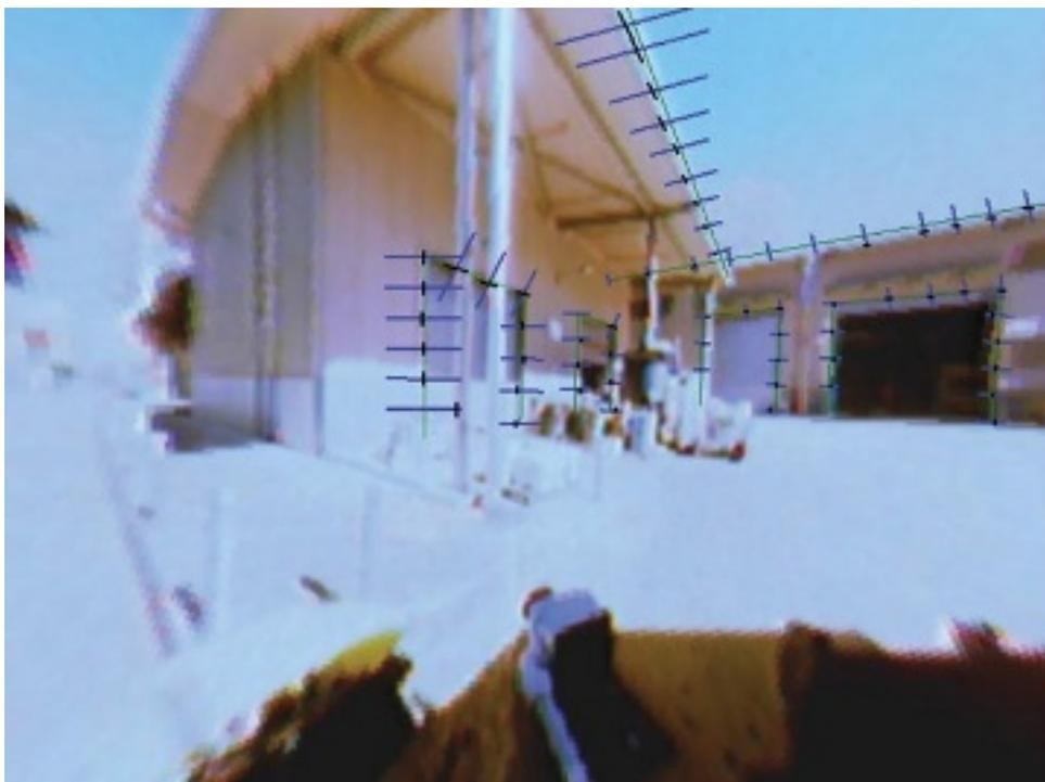
**Figure 3.** Nearest-edge search. The largest lines are the projected edges, the smaller perpendicular lines are the search along the edge normal, and the smallest lines indicate the nearest detected edge.
