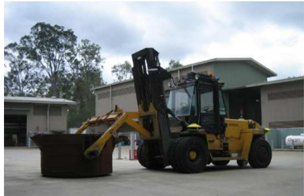
Fig. 1. A Hot Metal Carrier in the process of picking up the crucible of aluminium.
