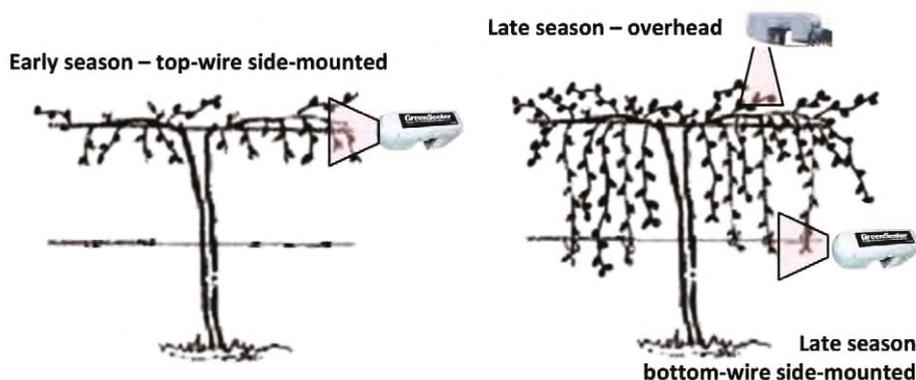
Figure 1. A schematic diagram of the orientation of the sensor relative to the canopy early and late in the season.
